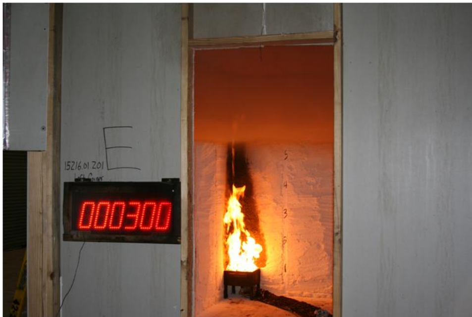
Figure 2. Burner at 40 kW: 3 min into Test.
