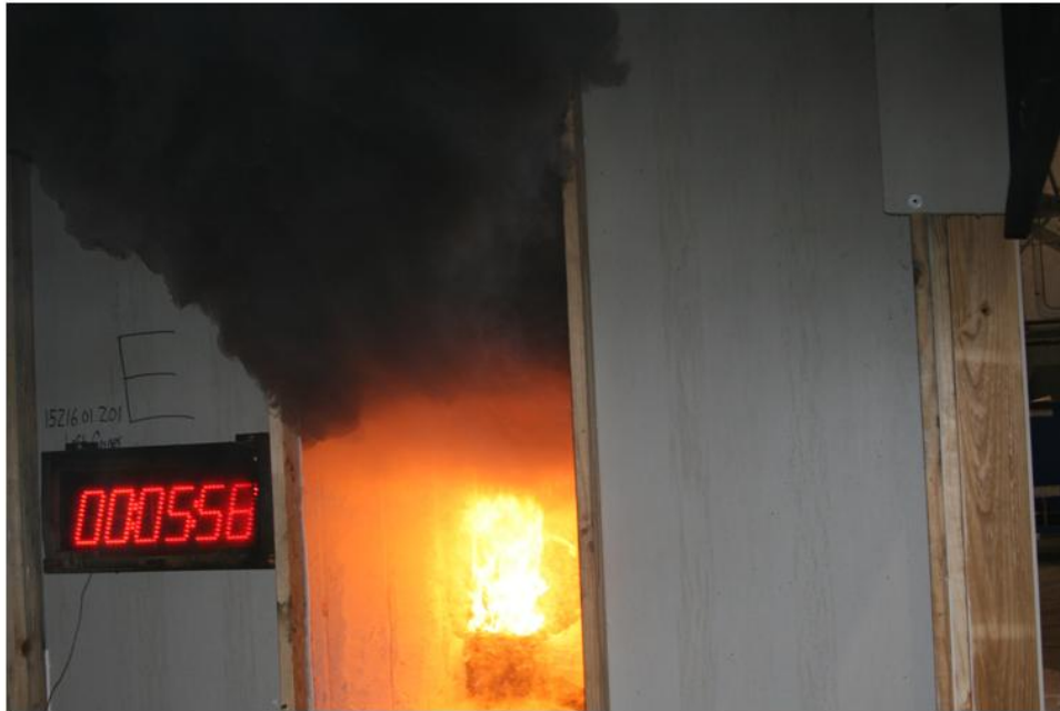
Figure 3. Burner at 160 kW: 5 min 56 s into Test.
