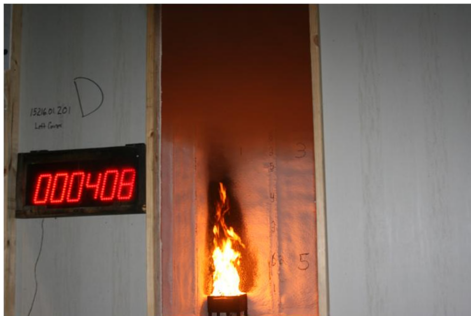
Figure 2. Burner at 40 kW: 4 min 8 s into Test.
