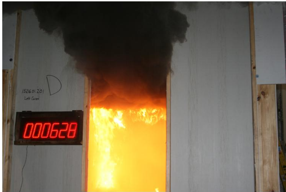
Figure 3. Burner at 160 kW: 6 min 28 s into Test.
